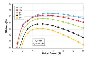
Figure 5. EPC9205 efficiency vs. output current for 48  $V_{\rm IN}$  to 5 -12  $V_{\rm OUT}$ when operating at 500 kHz and using EPC2045 eGaN FETs
