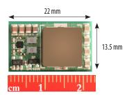
Figure 2: EPC9205 development board boasts a power density of 1400 W/in<sup>3</sup> when operating at 48 V input, 12 V output at 10 A load
