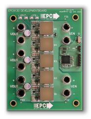
Figure 7: EPC9130 five-phase board with 12 A per phase has a maximum output current of 60 amps, making the board capable of over 700 W
